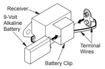
Figure 34 - Attaching Alkaline Battery to Receiver
